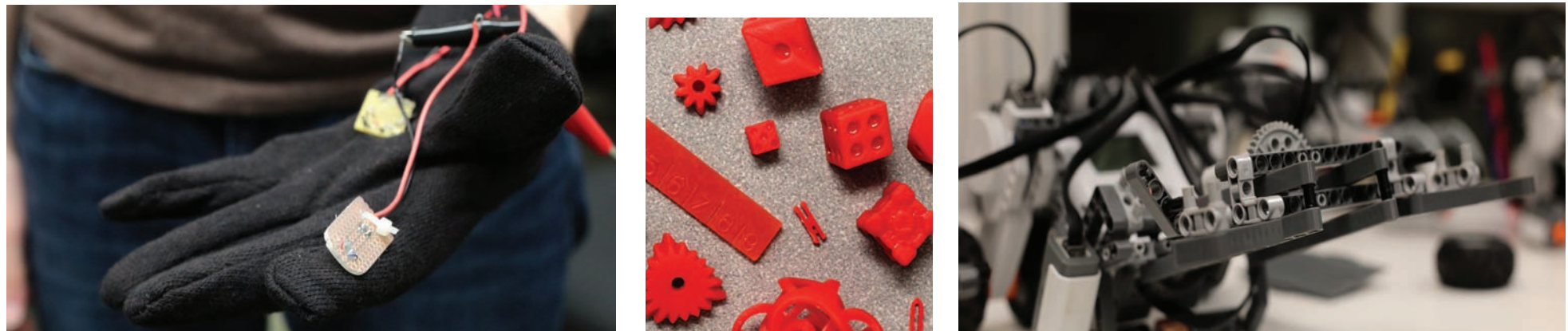
(Left to right): Haptech glove allows users to feel virtual reality; red bits manufactured in UR Robotics' 3D printer; Legos are used to test the mechanical soundness of prototypes. COURTESY OF BENNETT NIDENBERG
